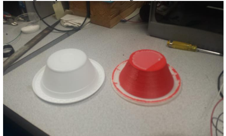
Fig 10. The object on the left is the original and the object on the right is the print out of our scan.
